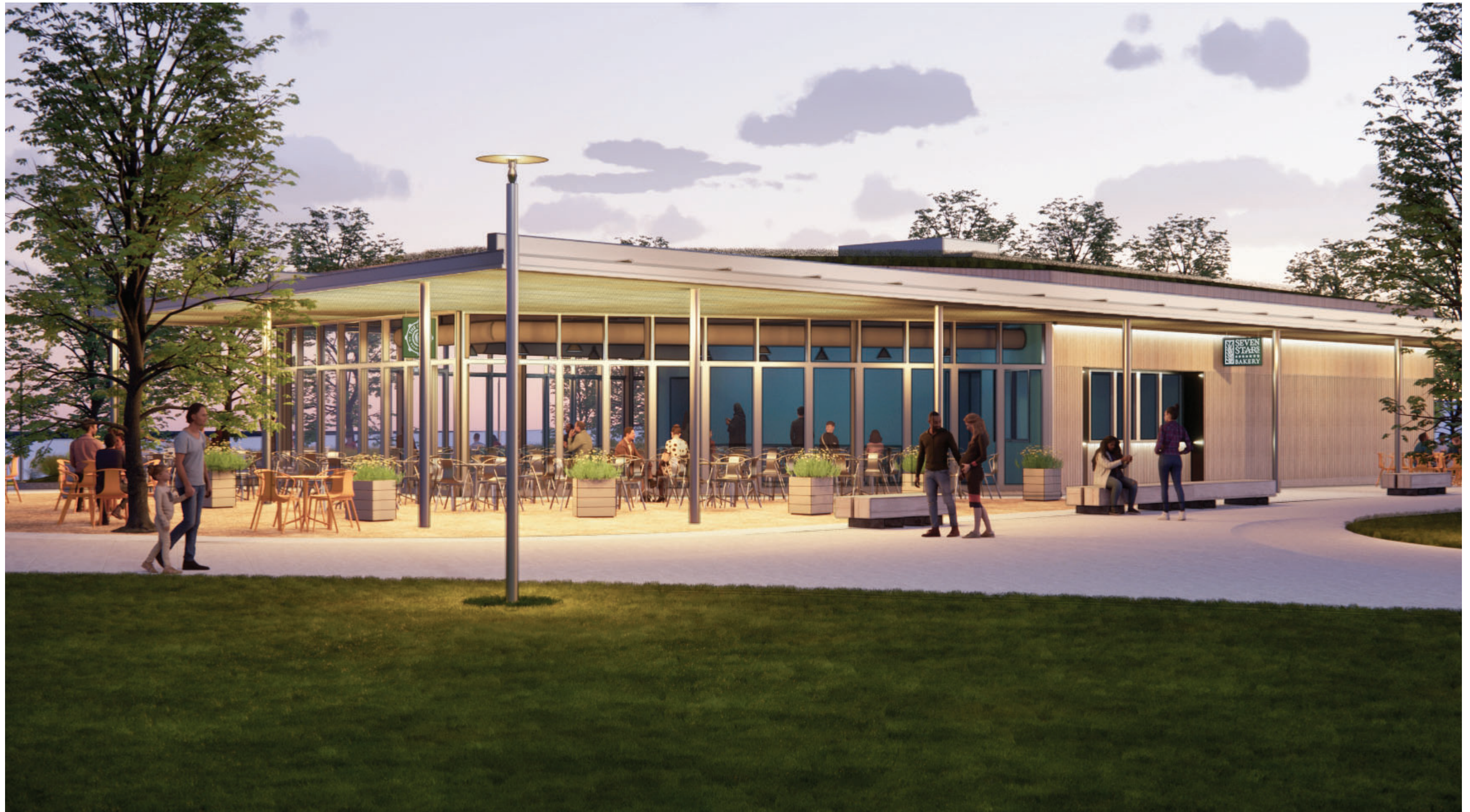
Twilight view from north park lawn facing south west. In-ground up lights wash the storefront structure with light. Wall grazers integrated in the exterior wall assembly accent the cedar siding.
